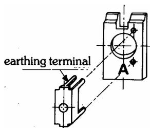
coding lugs part on the relay
